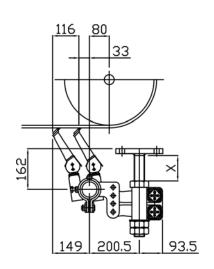
"X" = the tensile axis, the length must be at least 90 mm.
